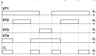
Obviously, the asymmetrical control makes it possible to reduce the current ripple without modifying the switching frequency.
