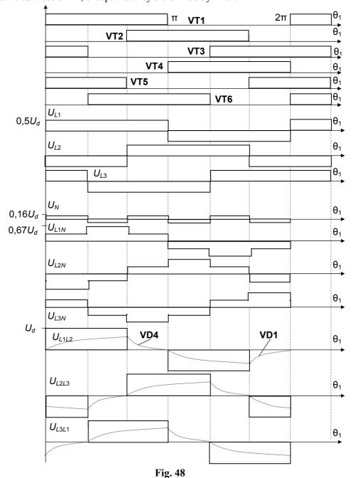
**Voltage-current analysis.** The rms value of the line-to-neutral voltage of the load for the described operation depends on the dc link voltage. This voltage can be expressed as
