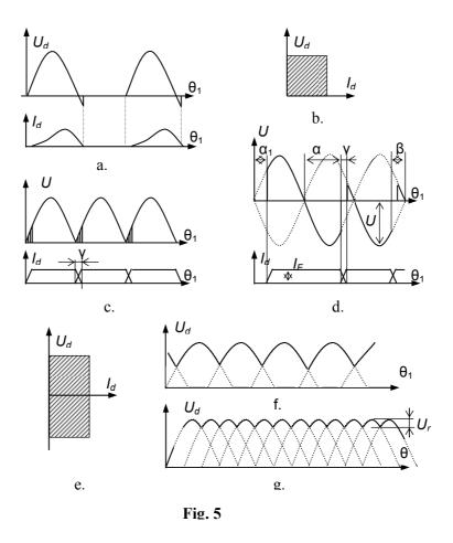
**Single-phase rectifiers.** At power levels below a few kilowatts, for example in residential applications, the loads are supplied by a single-phase supply source. Commonly used simple half-wave *single-phase rectifier* circuits (M1) are represented in Fig. 4, *a*, *b*. The resulting output *voltage* and *current* waveforms of the half-wave diode rectifier are shown in Fig. 5, *a*. Here
