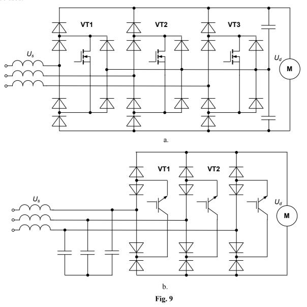
There is one controllable switch per phase: MOSFETs are depicted. Together with the surrounding four-diode bridges, they operate as bi-directional switches. When turned on, they connect the respective mains phase to the dc center point via the two diodes and the inductor, which makes the letter magnetize. When turned off, the inductor demagnetizes into the dc load through the freewheeling diodes connected to the positive and negative load terminals, respectively.
