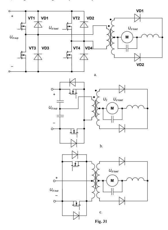
The midpoint converter shown in Fig. 31, *b*, consists of only two transistors but requires two split capacitors to form a dc input midpoint. It is sometimes used at slightly lower power levels compared to the full-bridge converter.
