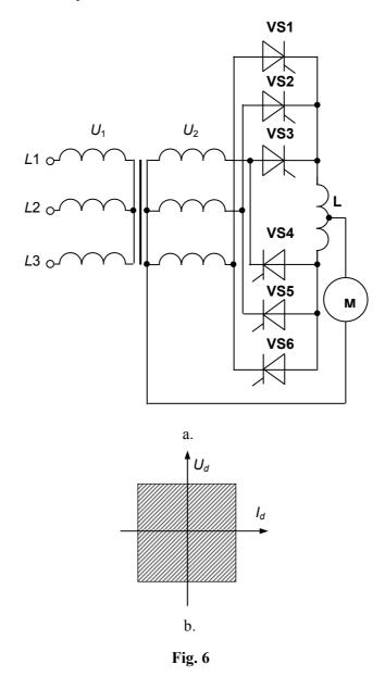
In Fig. 7, the anti-parallel connection of the two bridge rectifiers has been arranged to provide the four-quadrant operation. Such circuit is by far the most common industrial four-quadrant dc system and is used in many demanding applications where rapid control is required. Usually, they incorporate additional features to enhance the safety of operation and to improve the control transients.
