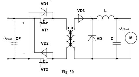
The bridge transformer-isolated buck converters provide two-quadrant operation using the center-tapped transformer with the magnetic core. In Fig. 31, a, voltage applied to the primary winding alternates without a dc component. The waveform of this voltage has equal positive and negative volt-seconds, although the load voltage is always of a dc shape.
